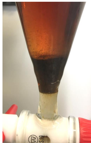
Adding petroleum ether: Sludge does not mix with other phases
