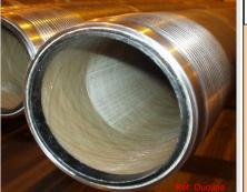
—C steel -CS + Inhib -GRE lined -DSS 10 ( GRE lined tubing Smillion higher initial CAPEX vs carbon steel or carbon Costs steel + corrosion inhibitor, but surpassed 2 after year 3-6 plus fewer workovers -ADNOC Onshore 15 10 20 Year 25 tested in disposal well
