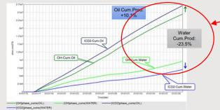
2. Well optimized design with ICD liner giving >10% cumulative oil & 24% less water versus open hole
