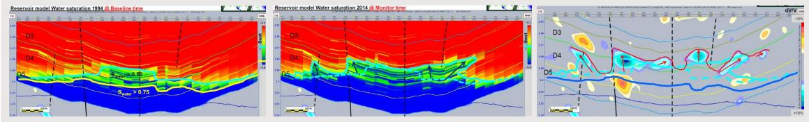
Water saturation over time monitored by 4D seismic to compare against reservoir – ADNOC Offshore example of comparison of reservoir model to seismic
